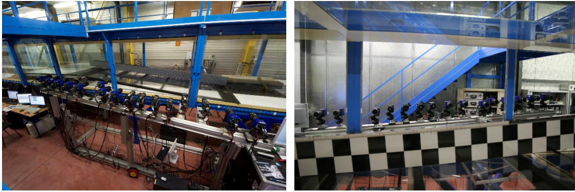
Figure 8: Set of 16 sCMOS cameras mounted on the side of the wind tunnel. The target used for calibration is visible in the right image.
