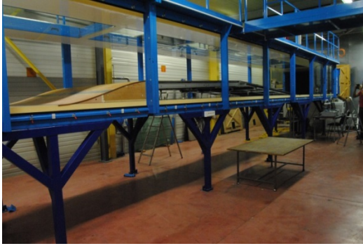
Figure 4: Test section of the LML wind tunnel with EuHIT model mounted on the floor.
